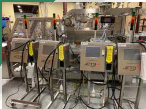
4 Head CIJ Printer needs 4 Controllers
