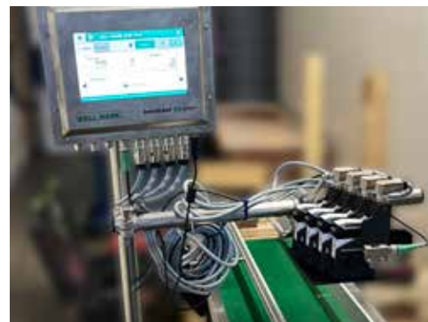
4 Head TIJ Printer needs 1 Controller
